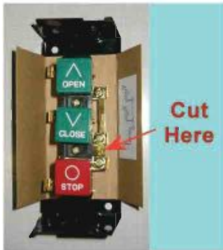
Photo #32 (NEMA-1 Station Cut Point)
