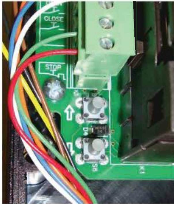
Photo #26 (Manual Override Buttons)
