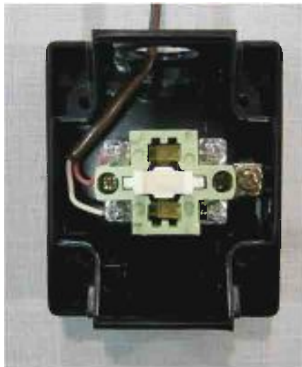
Photo #36 (Single Button Station Wiring)
