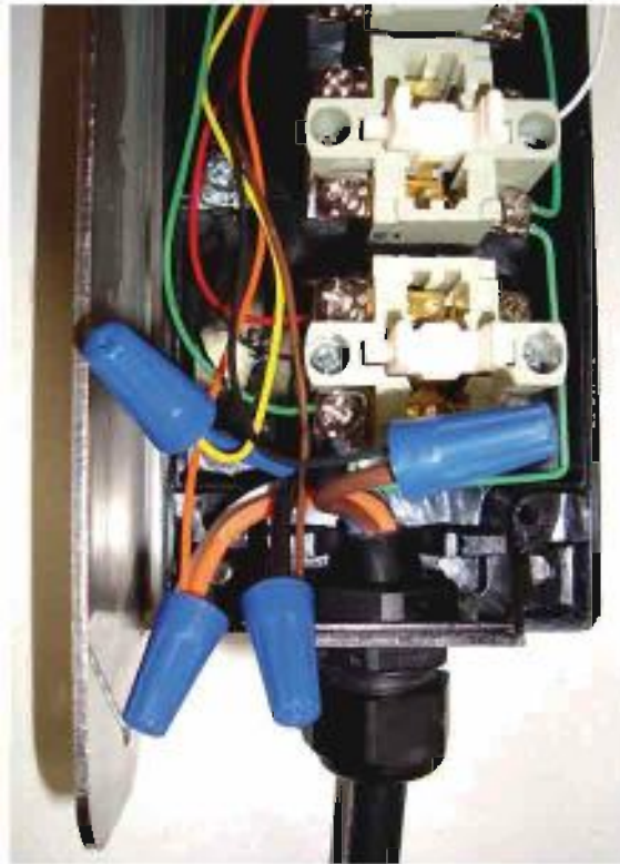
Photo #22 (Safety Edge Wire Nuts)
