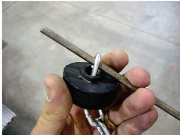
Photo #11 (Stop Bumper Installation)
