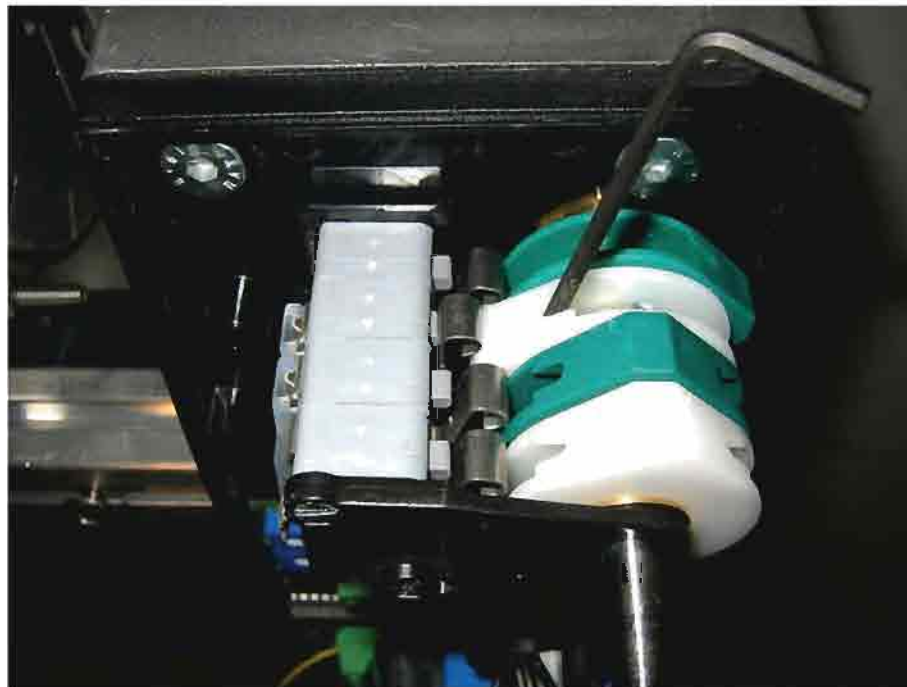
Photo #27 (Cam Phase Screw Adjustment)
