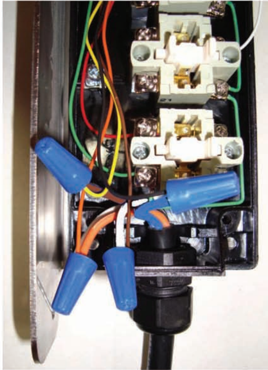
Photo #22 (Safety Edge Wire Nuts)
