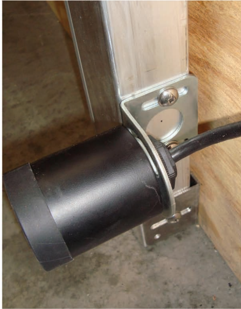
Photo #7 (Head Unit Mounting)
