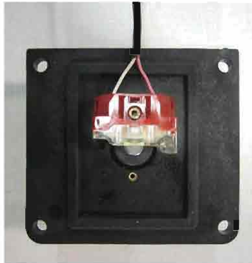
Photo #37 (Pullcord Switch Station Wiring)
