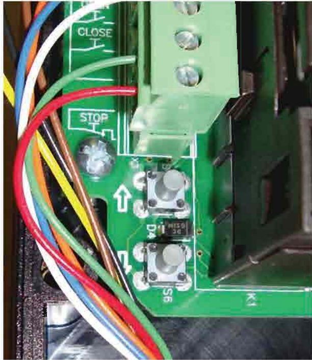
Photo #26 (Manual Override Buttons)
