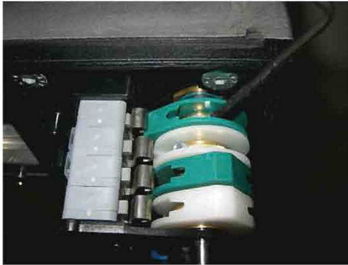
Photo #11 (Open Cam Coarse Adjustment)
