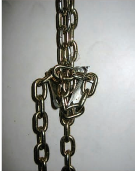
Photo #15 (Hoist Chain Locking)
